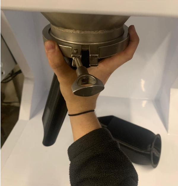
5. Orient the head direction and tighten the tri-clamp:
