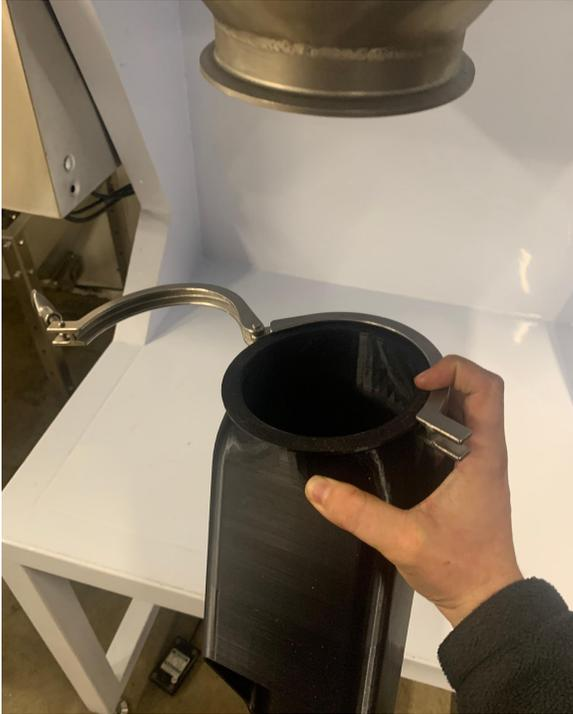
3. Place the tri-clamp around the flange on the desired head:
