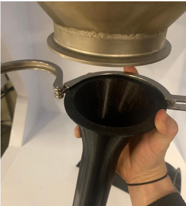
4. Slide the head and tri-clamp onto the outlet:
