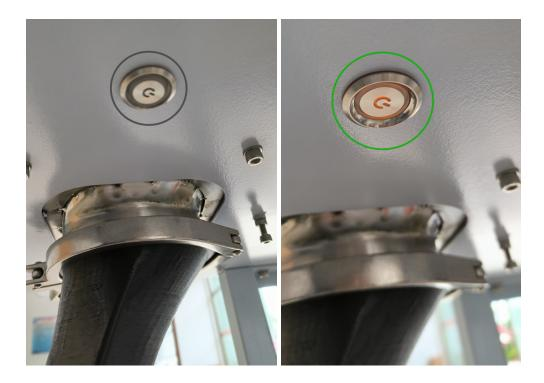
4. To power off the machine, simply press the power button again.
