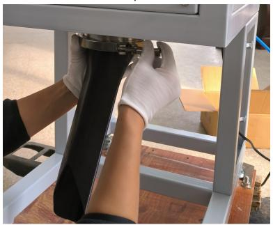
5. Orient the head direction and tighten the tri-clamp:
