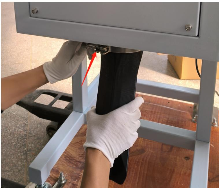
2. Slide the tri-clamp and head off of the outlet:
