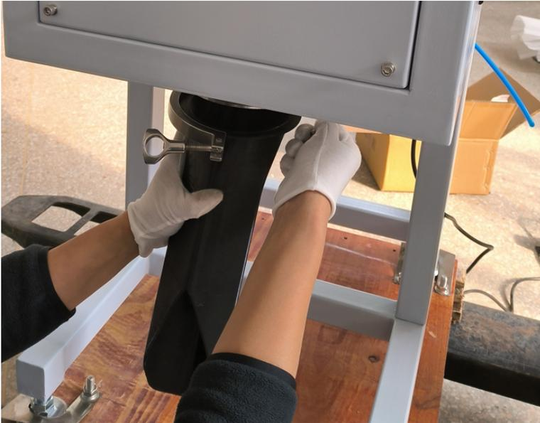
3. Place the tri-clamp around the flange on the desired head:
