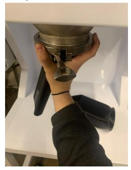
5. Orient the head direction and tighten the tri-clamp:
