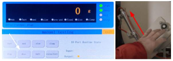
2. fast [Fast Feed Button]: When you tap the Fast Feed button, the filling gate should be all the way open and the vibrator should be operating.
