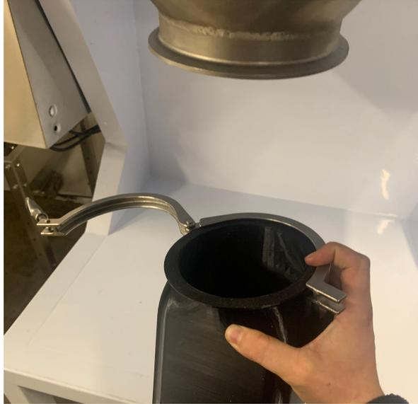
3. Place the tri-clamp around the flange on the desired head:
