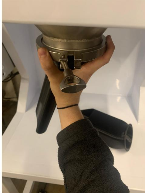
5. Orient the head direction and tighten the tri-clamp:
