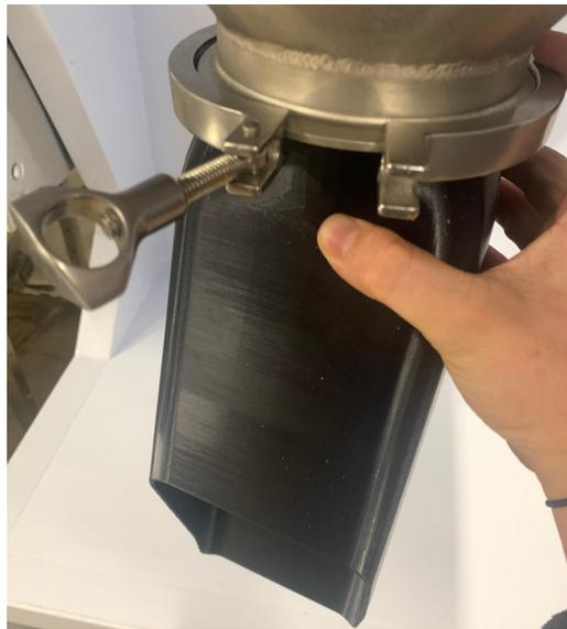
2. Slide the tri-clamp and head off of the outlet:
