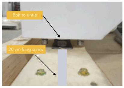
5. If hex head machine screws are inserted in the feet of the body, remove those and put them in a convenient location you can access later.
