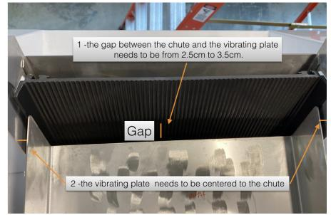
a. If you don't have 2.5cm to 3.5cm you will need to loosen the 4 screws at the base of the vibrator plate so the vibrator can be adjusted. Do not fully remove the screws, or the bolt plate they attach to will drop into the machine. Simply loosening them slightly will be sufficient.
